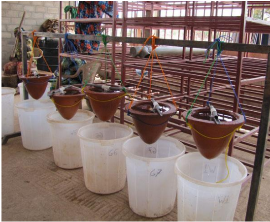
Figure 74: Flow test rack
