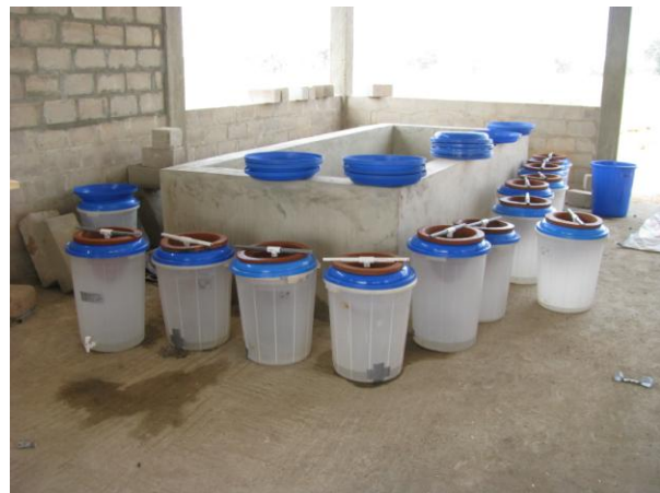
Figure 61: Filter flow rate tests
