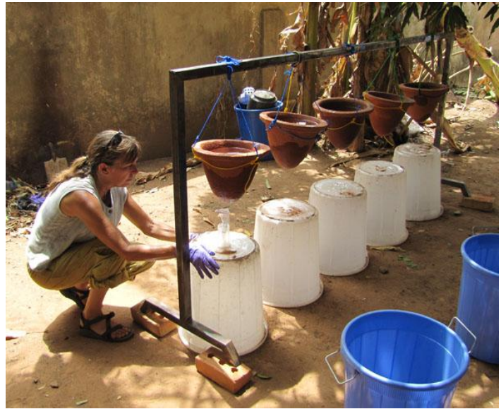
Figure 67: Collecting water samples directly from filter into Whirl-Pak® bag outside of Kalpohine office (Source: Bradner)
