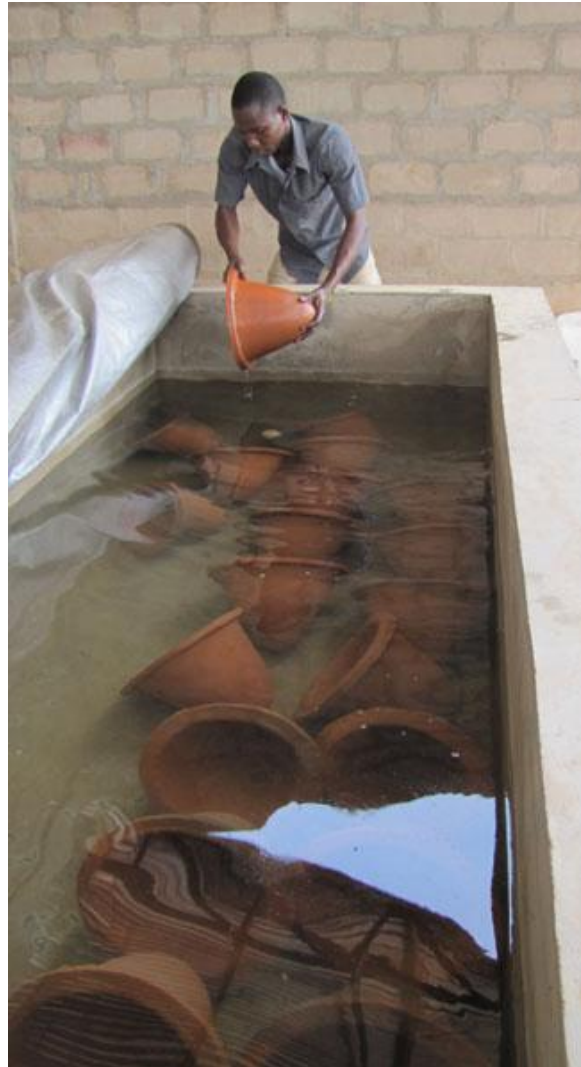
Figure 77: Karim bubble tests filters
