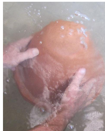
Figure 70: Bubble test – failed filter (Courtesy of Bradners)
