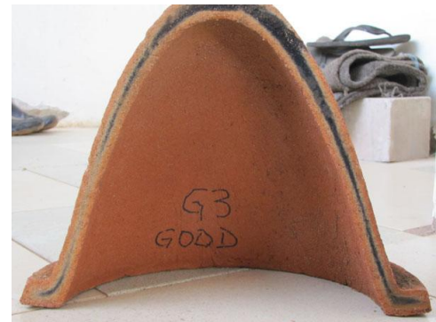
Figure 68: Under-fired filter (Source: Bradner)
