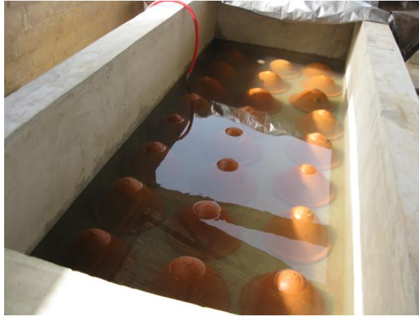
Figure 55: Filters soaking in the saturation tank
