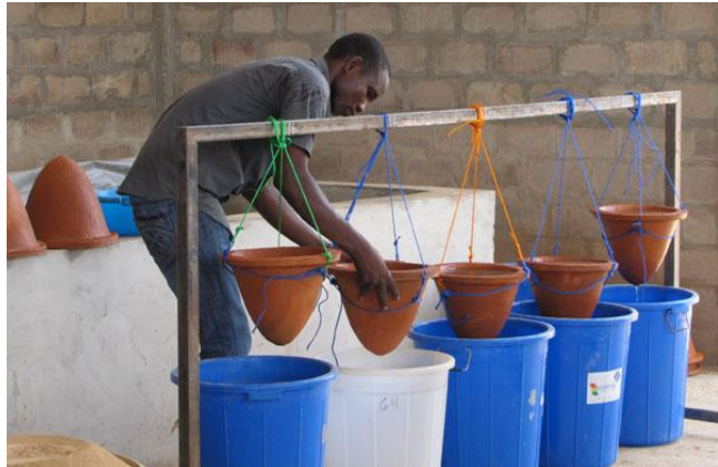
Figure 75: Karim Flow Tests Filters
