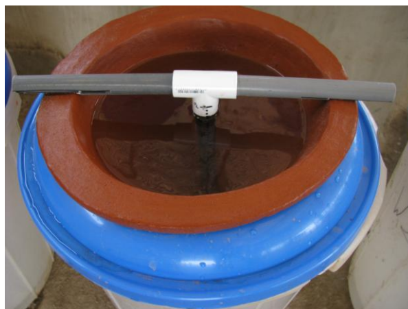
Figure 62: T-device in filter element for flow test
